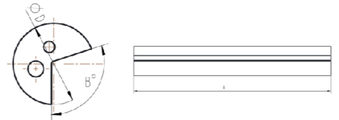
带槽双孔型/ Profile rods with two coolant holes
